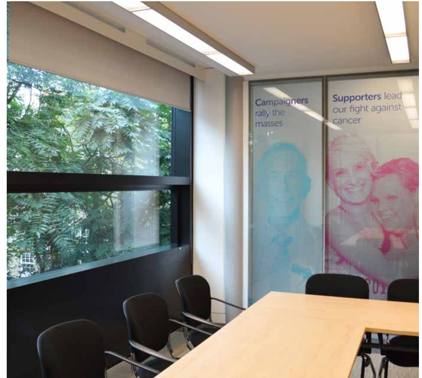
Printed optically clear window film applied to all internal windows in one of the large boardrooms and dusted film applied to the other side of the glass.
